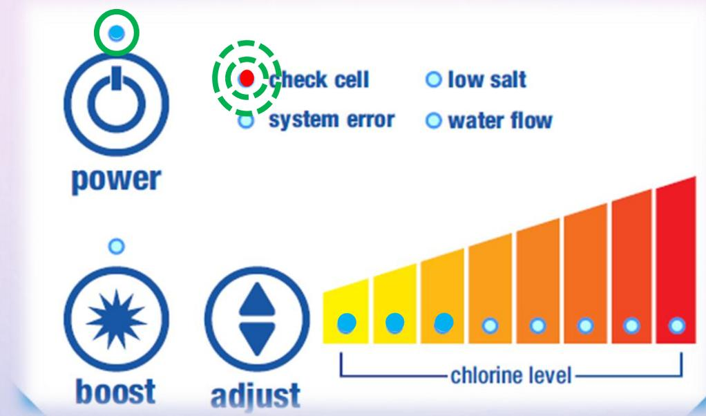
Check Cell Light Flashing is a timed warning that the cell has been running for 8,000 hours. This serves as a reminder to clean the cell if it has not been cleaned recently. At this point, it is advisable to check amps and volts using the Tech Mode procedure reviewed on the previous pages. If the amps and volts are in range, the cell is functional to continue operation. The PSU will need to be reprogrammed to clear the flashing check cell indicator.
