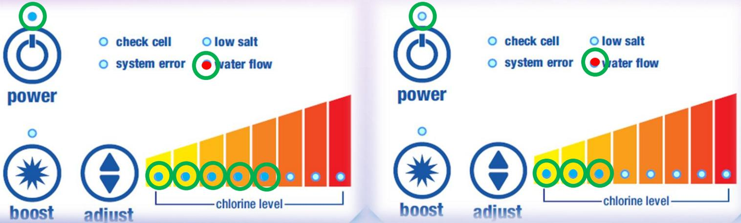
**Example shows 5 lights LIT with ON/OFF LED ON and 3 lights LIT with ON/OFF LED light OFF; tech mode reporting 5.3 amps**
