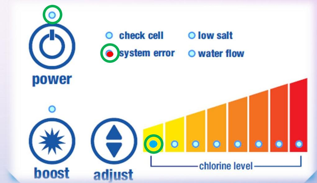
*If none of the above resolve the System Error 1, proceed with the further troubleshooting on the next page to determine the second numerical error code for the System Error one. (Example: System Error 1.1, System Error 1.2, and so on).*
